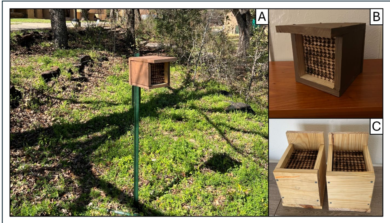
Figure 2. Images of bee box design (A) adhered to a t-post at site WL, (B) after being painted with wood stain, and (C) in the early phase of construction
